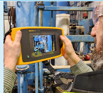
Partner checking for compressed air leaks using an ultrasonic leak detector.
